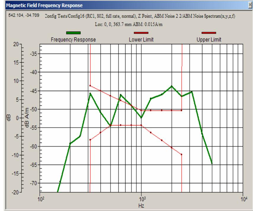
RC1, SO2, vocoder rate full, normal laboratory background noise
